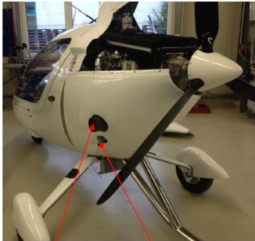
Intake after modification
